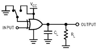
C<sub>L</sub> includes load and stray capacitance
